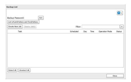
4 Check the IP address of the LinkStation or TeraStation that you want to set as the backup target. Click *Add*, enter the IP address of the target LinkStation or TeraStation, and click *Close*.
