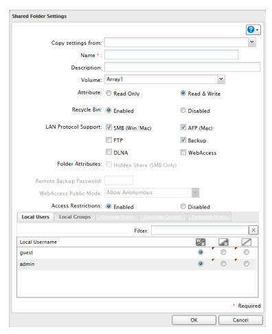
**Note:** To configure a password, enter it in the "Remote Backup Password" field. Leave this field blank if you don't want a password. If the target device is configured with a backup password, you can search for the password from the backup source.
