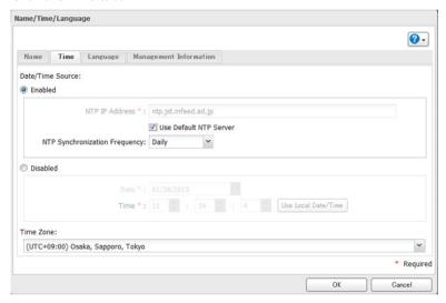
By default, the LinkStation adjusts its clock automatically by using a default NTP server.
